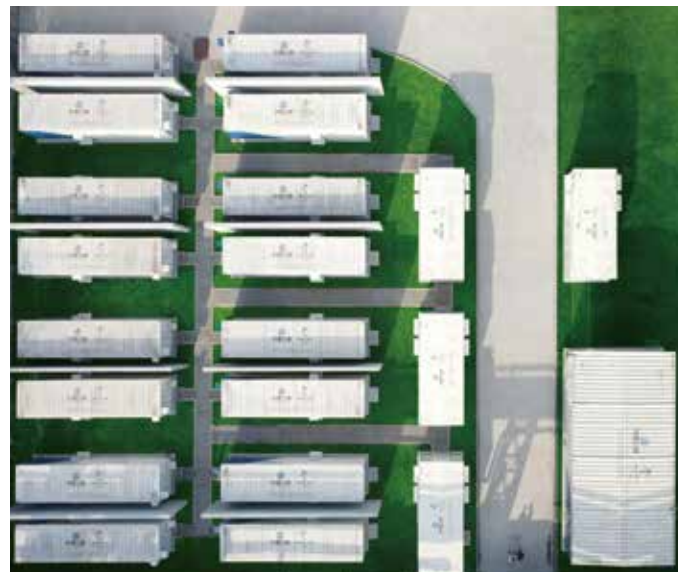
Jiangsu Steel Plant Energy Storage Power Station Power Capacity: 10MW/39MWh
